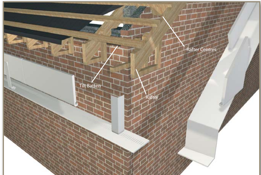
Fig 1. Framing out for New Build/Full Replacement installation. Illustration showing the rafter centres, the support soffit bearer/tilt batten across rafter feet, and fascia board showing the fixing points.
