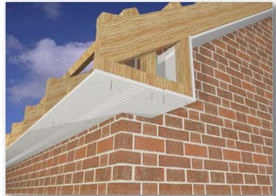
Fig 9. Typical GPBV soffit installation.
