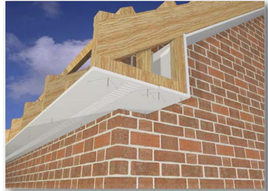
Fig 20a. Typical GPBV soffit installation.
